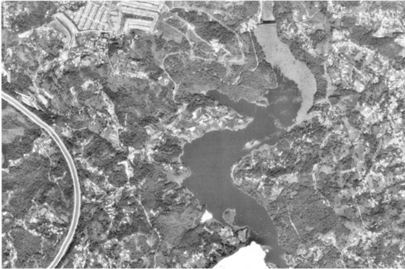
Fig. 3. Aerial view of the northern section of the Loíza reservoir and dam, Puerto Rico, 1991, showing high degree of landscape development, including housing, commercial buildings, secondary road, and expressway. Light gray area on reservoir surface behind dam is a floating mat of water hyacinths ( Eichhornia crassipes ). Dam measures 210 m across top.
