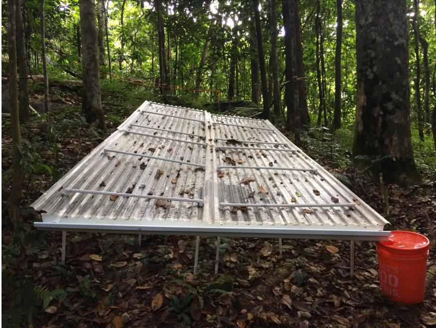
*Fig. 4. Photograph of throughfall exclusions being used to experimentally test the effect of drought on soil biogeochemistry and litter/soil organisms.*
