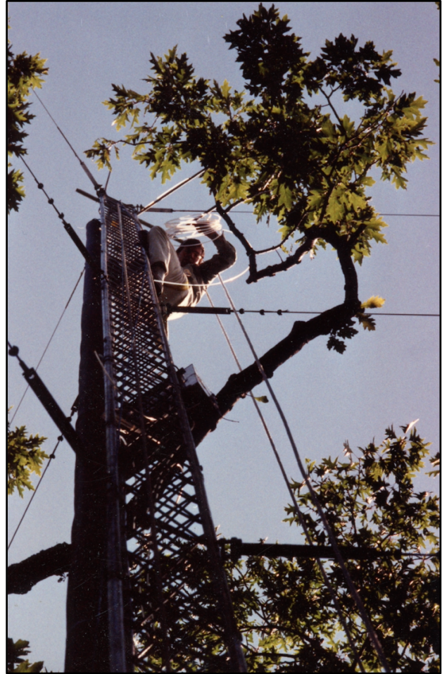
Bill setting up a large metal tower in Harvard Forest in 1989, used to measure long-term CO 2 exchange.
